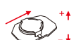
4. Input the new battery (please note the positive and negative polarity of the battery)
